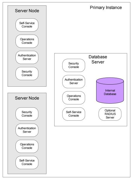
The Security Consoles shown on the server nodes receive requests distributed by the proxy service on the primary database server. In a typical configuration, browser access to the Security Console is directed to this proxy service at port 7004 on the primary instance database server.
