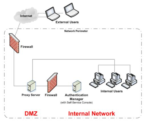
The following figure illustrates a basic network setup with Self-Service Console traffic directed through a proxy server.
