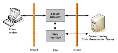
This diagram shows how the Secure Gateway secures communication between SSL/TLS-enabled clients and servers.
