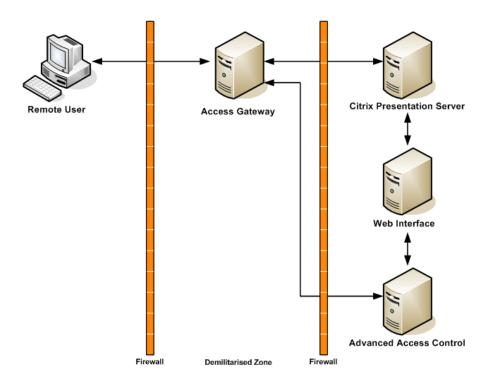
This diagram shows the recommended deployment for using Advanced Access Control with the Web Interface.
