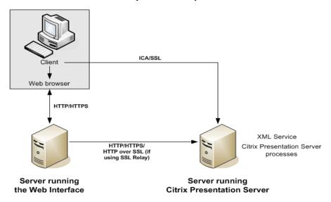
This diagram shows how the client device interacts with the server running Presentation Server and the server running the Web Interface.
