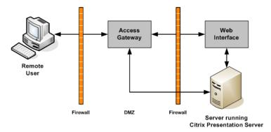
This diagram shows how the Access Gateway secures communication between SSL/TLS-enabled clients and servers.
